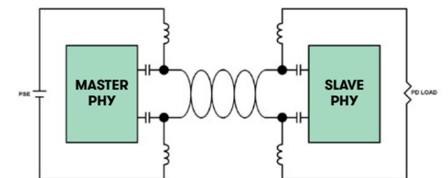
Fig. 5. Simultaneous transmission of data and power supply via the cable pair. (Fig.: channel-e)
