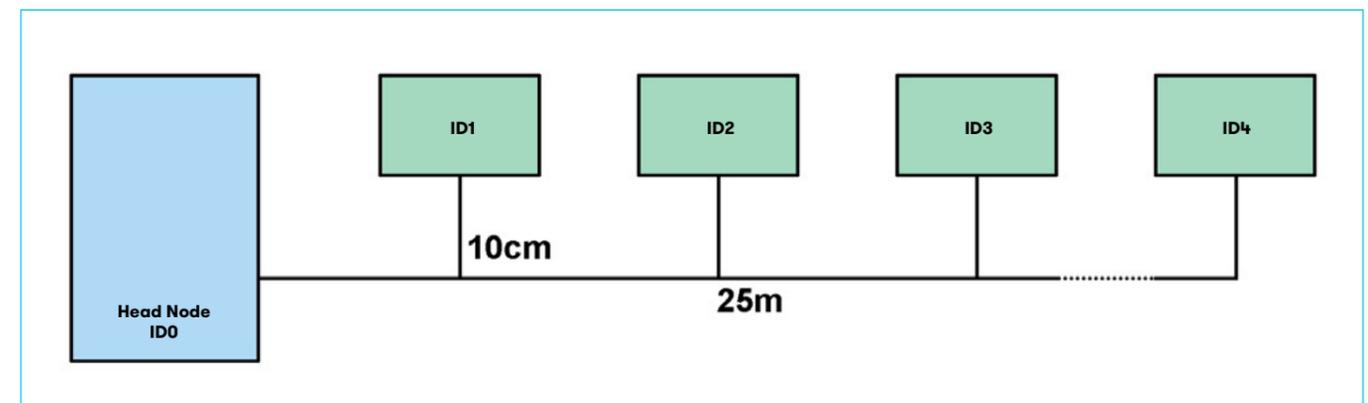
Fig. 1. 10BaseT1S works in the half-duplex process and is operated in a multi-drop technology, which defines a bus length of 25 m with 10 cm-long stubs. (Fig.: channel-e)
